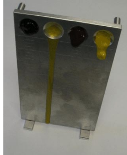
FP-4-5GM Shown in vertical test position
