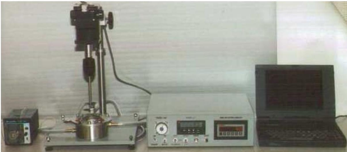
**OVERVIEW:** Kershaw Instrumentation L.L.C. has developed a technique for measuring water pickup of inks. This "titration" test is an automatic approach, which is quick and reproducible and requires no operator attention once the test is started. The digital displays on the instrument console eliminate the requirement of evaluation and/or analysis of the data by the operator, thus eliminating operator error.
